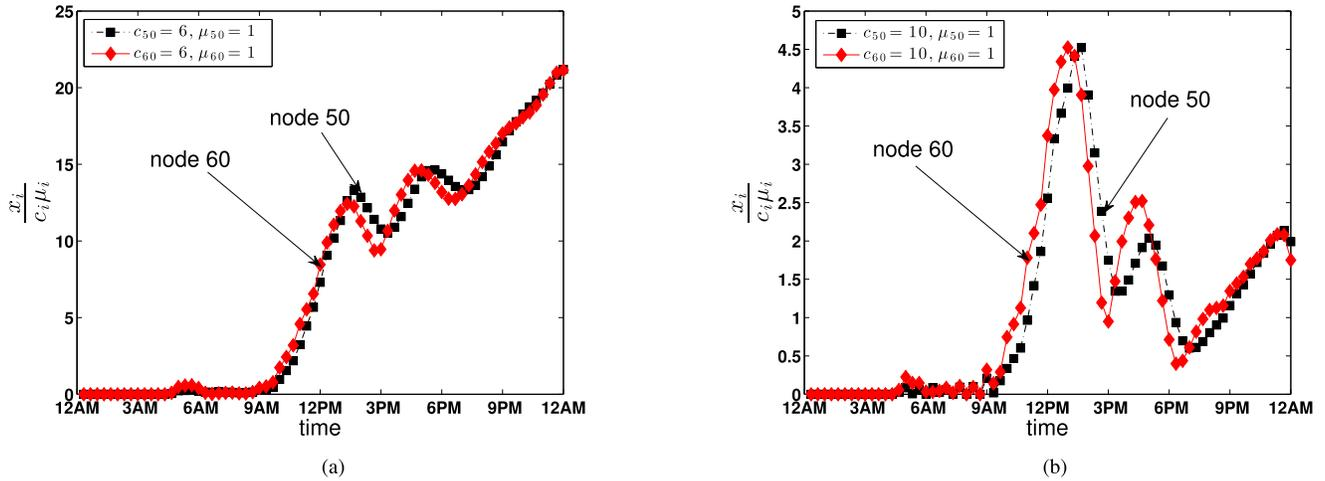
Fig. 15. Utilization of service stations for real Florida turnpike data with  $\mu_{50} = \mu_{60} = 1$  EV/h. (a)  $c_{50} = c_{60} = 6$ . (b)  $c_{50} = c_{60} = 10$ .
