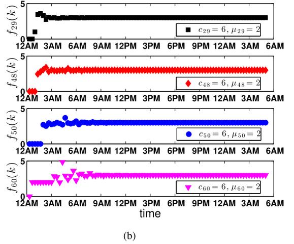
Fig. 8. Simulation results under the proposed consensus-based scheduling algorithm for constant traffic flow  $\gamma_{14}(k) = 4$ ,  $\gamma_{36}(k) = 6$ ,  $\gamma_{54}(k) = 2$  with  $c_{29} = c_{48} = c_{50} = c_{60} = 6$  and  $\mu_{29} = \mu_{48} = \mu_{50} = \mu_{60} = 2$  EVs/h. (a) Utilization of service stations. (b) Number of EVs entering service stations.
