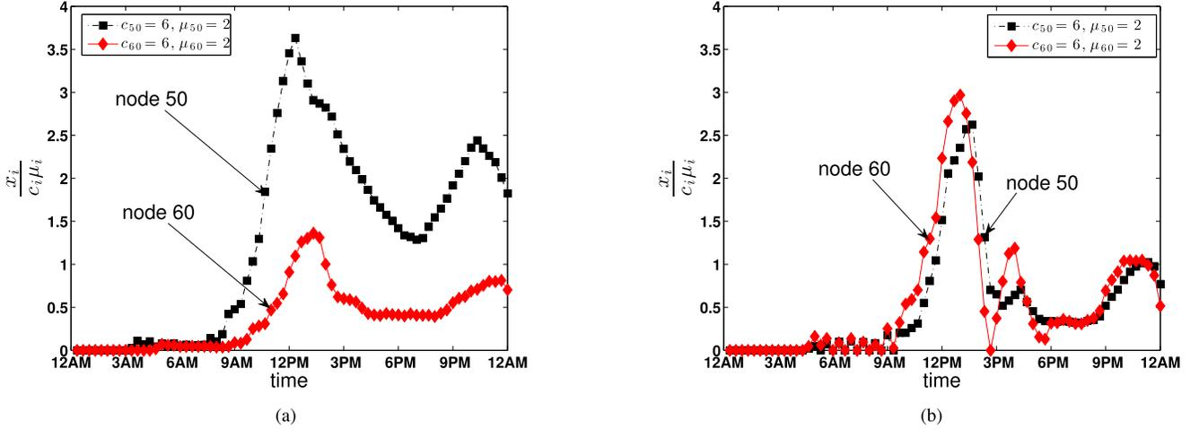
Fig. 12. Utilization of service stations for real Florida turnpike data with  $c_{50} = c_{60} = 6$  and  $\mu_{50} = \mu_{60} = 2$  EVs/h. (a) SoC-based random charging strategy. (b) Consensus-based scheduling algorithm.
