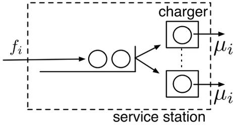
Fig. 3. A queuing model for service station at node  $i$ .
