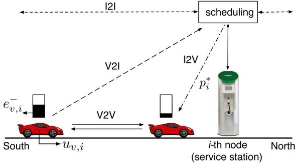
Fig. 5. Distributed scheduling and cooperative control of EVs using infrastructure-to-infrastructure (I2I), vehicle-to-vehicle (V2V), vehicle-to-infrastructure (V2I) and infrastructure-to-vehicle (I2V) communication.
