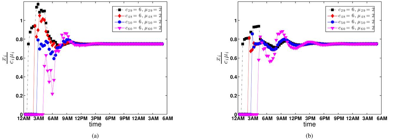
Fig. 10. Simulation results under the proposed consensus-based scheduling algorithm for different communication topologies and constant traffic flow  $\gamma_{14}(k) = 12$  with  $c_{29} = c_{48} = c_{50} = c_{60} = 6$  and  $\mu_{29} = \mu_{48} = \mu_{50} = \mu_{60} = 2$  EVs/h. (a) Consensus-based algorithm for topology in figure 9a. (b) Consensus-based algorithm for topology in figure 9b.
