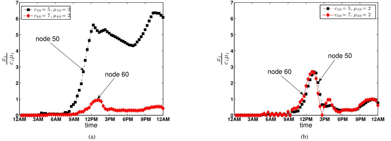
Fig. 13. Utilization of service stations for real Florida turnpike data with  $c_{50} = 5$ ,  $c_{60} = 7$  and  $\mu_{50} = \mu_{60} = 2$  EVs/h. (a) SoC-based random charging strategy. (b) Consensus-based scheduling algorithm.
