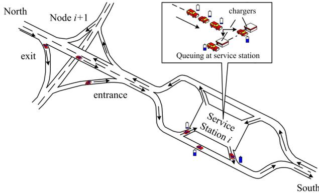
Fig. 1. A bidirectional highway segment with exit/entrance and service station.
