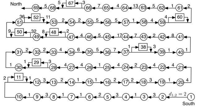
Fig. 7. The map of entrances/exits and service stations on Florida Turnpike. The circles represent entrances/exits and the rectangles represent service stations. The numbers above the arrows represent the distance (in minutes increments) between two consecutive nodes and the numbers in the circles denote the label of the entrances/exits and service stations.
